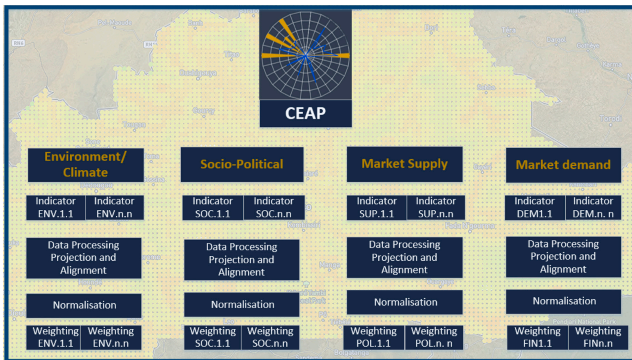
Fig. 2. Structure of the Clean Energy Access Prioritiser Index determined per planning unit (depending on user weights).
